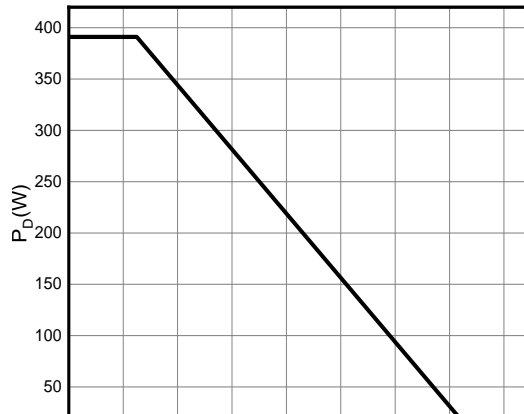
Figure 12. Power Dissipation vs. Temperature
